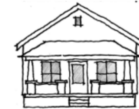
Bungalow Characteristics: · Low-pitched roofs · Characterized by simple living · Porch may or may not be beneath main roof extension
