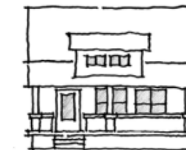
Craftsman Characteristics: · Low-pitched roofs with deep overhangs · Porch beneath main roof extension · Exposed rafters and knee brackets
